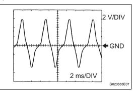
Check the waveform between terminals NT+ and NT- of the ECM connector. **Standard:**
